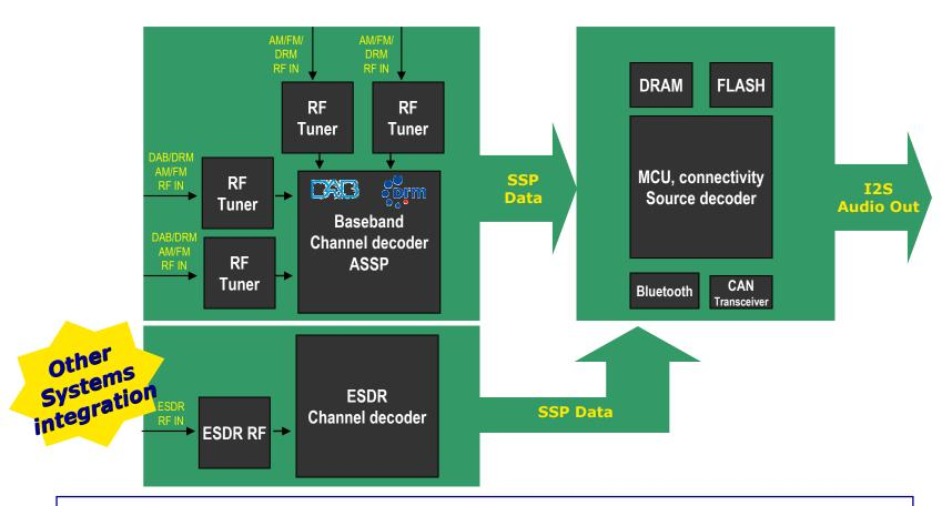
High complexity (i.e. ESDR) or proprietary systems may not be easily and efficiently integrated into multi-standard chip solution.
