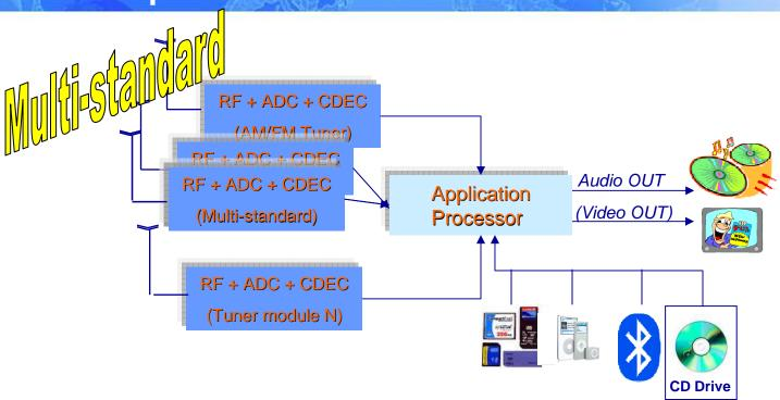
This partitioning allows a simple and efficient evolution versus multi-standard chip for the digital radio receivers
