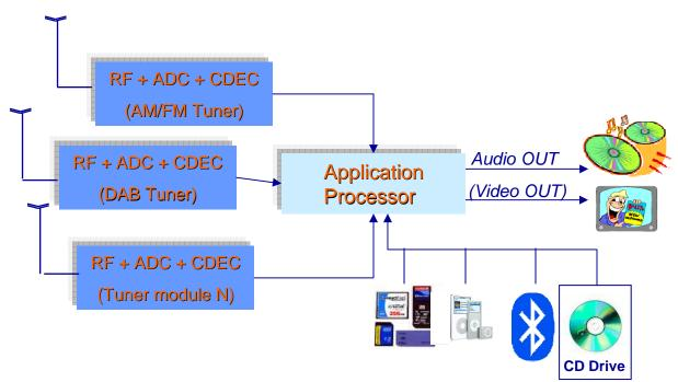
Tuner module(s) including RF and channel decoder ASSP + Application Processor for source decoding and connectivity
