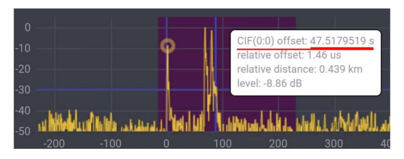
Channel Impulse Response where all three transmitters (three yellow peaks), work within the guard interval of 246µs
