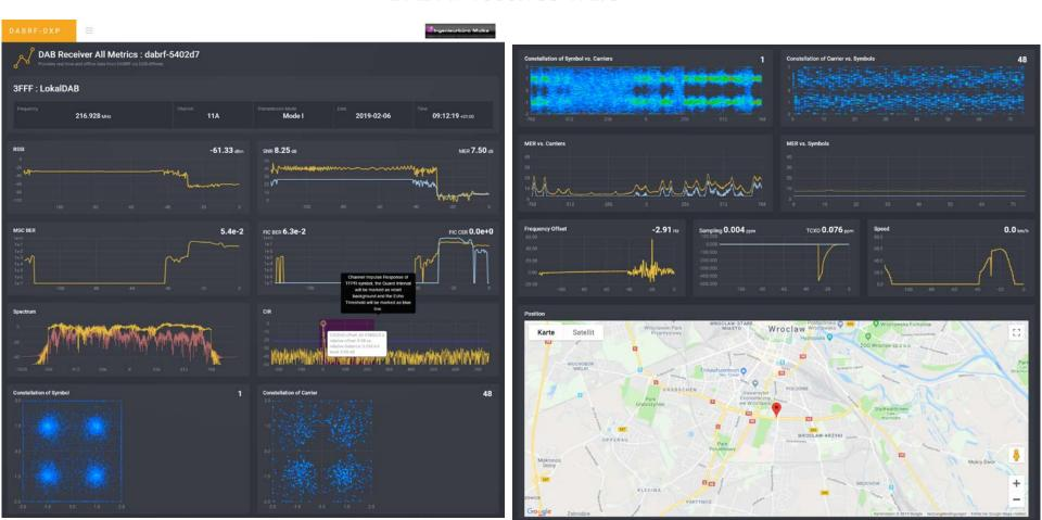
In both cases the RF level is around -62 dBm, which is high enough for a good reception, but the SNR is 8 dB which is very low.
